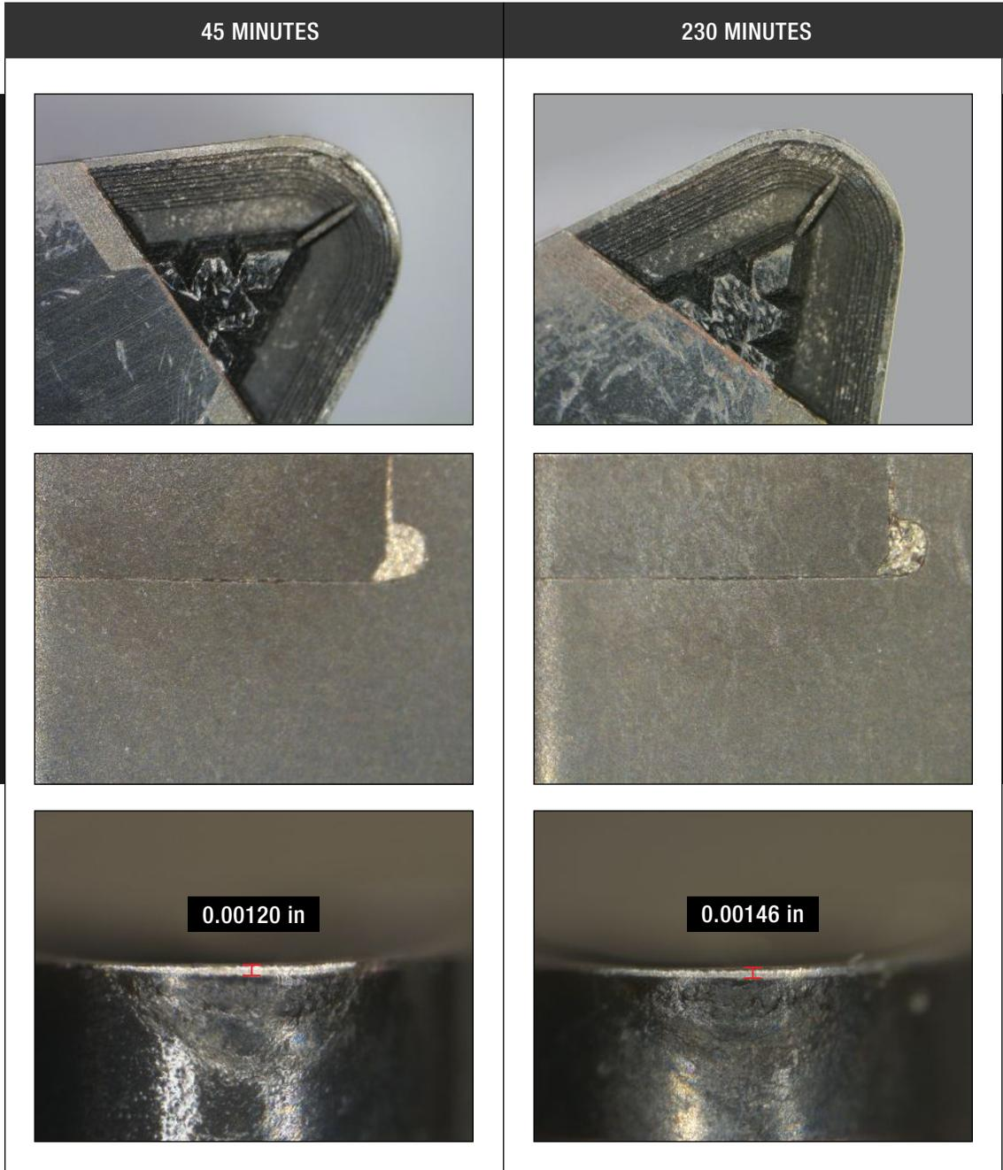
At 400 sfm (twice the speed of carbide) and 230 minutes in the cut, the binderless CBN insert was still performing consistently. The carbide insert required indexing at the 45-minute mark.
